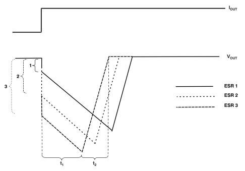
Figure 24. Correlation of Different ESRs and Their Influence to the Regulation of V<sub>OUT</sub> at a Load Step From Low-to-High Output Current
