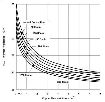
Figure 27. Thermal Resistance vs Copper Heatsink Area
