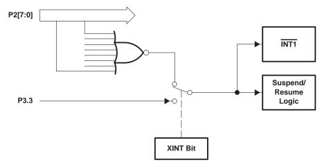
Figure 2–5. P2[7:0] Input Port Interrupt Generation
