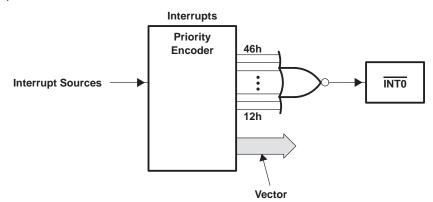
Figure 2–4. Internal Vector Interrupt (INT0)
