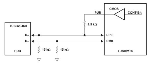
Figure 2–3. Pullup Resistor Connect/Disconnect Circuit
