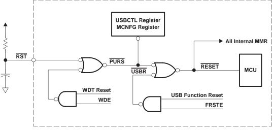
Figure 2–2. Reset Diagram
