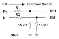
Figure 4–5. Downstream Connection – Only One Port Shown
