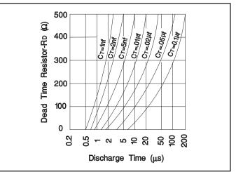
Oscillator Discharge Time vs R<sub>D</sub> and C<sub>T</sub>.
