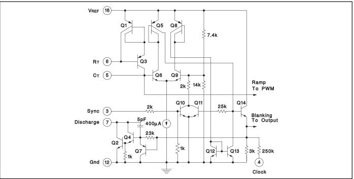
UC1525A oscillator schematic.
