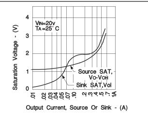
UC1525A output saturation characteristics.
