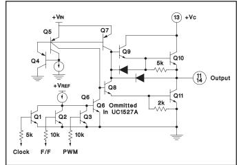
UC1525A output circuit (1/2 circuit shown).
