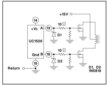
Figure 9. Driving N-channel Power Mosfets
