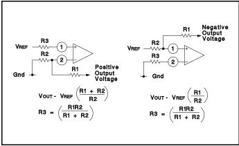
Figure 6. Error Amplifier Connections
