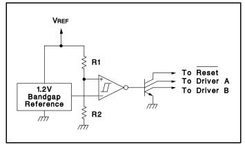
Figure 2. Under-Voltage Lockout Schematic
