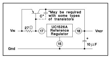
Figure 1. Extending Reference Output Current
