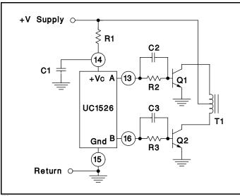
Figure 7. Push-Pull Configuration
