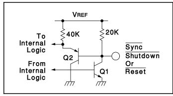
Figure 4. Digital Control Port Schematic
