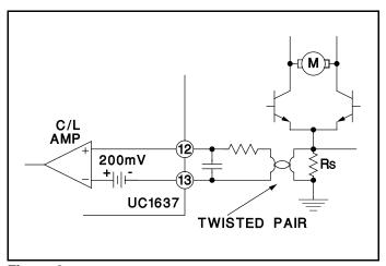
Figure 6. Current Limit Sensing
