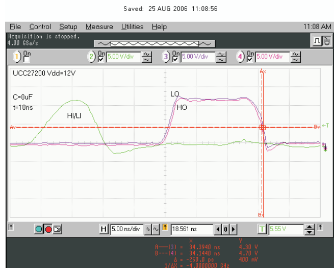
Figure 34. 10-ns Input Pulse Delay Matching
