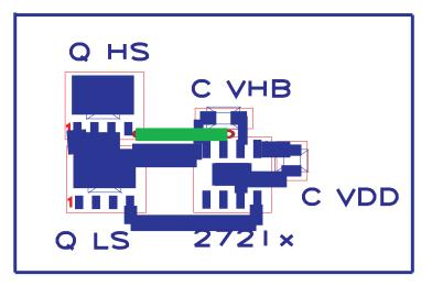
Figure 24. UCC27210/11 Component Placement
