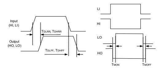
Figure 1. Timing Diagrams
