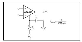
Figure 47. Control Line Filtering
