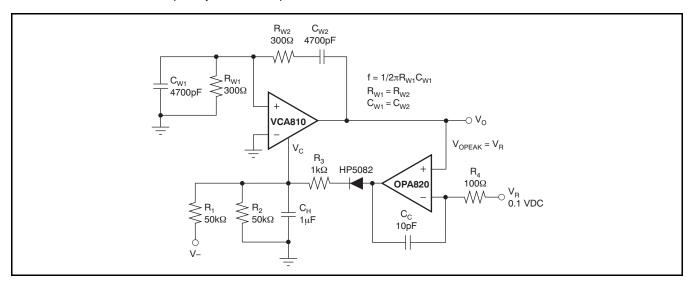
Figure 34. Amplitude-Stabilized Oscillator
