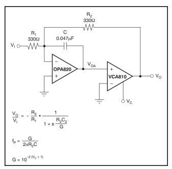
Figure 39. Tunable Low-Pass Filter
