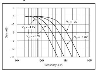
Figure 40. Voltage-Controlled Low-Pass Filter Frequency Response
