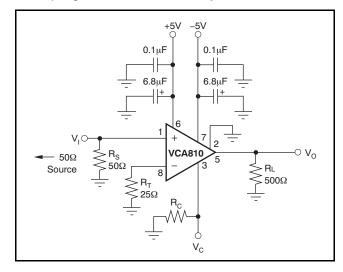
Figure 30. Variable Gain, Specification and Test Circuit
