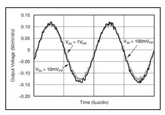
Figure 33. AGC Output Voltage for 100kHz Sinewave at 10mV<sub>PP</sub>, 100mV<sub>PP</sub>, and 1V<sub>PP</sub>
