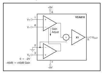
Figure 29. Block Diagram of the VCA810
