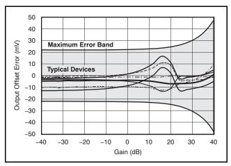
Figure 45. Output Offset Error versus Gain
