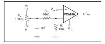
Figure 46. Optional Offset Adjustment
