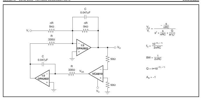
Figure 43. Tunable Band-Pass Filter
