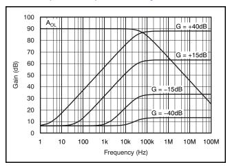
Figure 42. Amplifier Noise Gain and A<sub>OL</sub> for Different Gain
