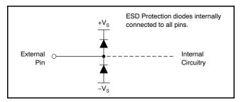
Figure 49. Internal ESD Protection
