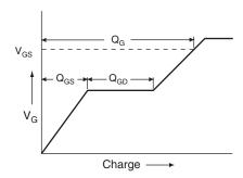
Fig. 13a - Basic Gate Charge Waveform
