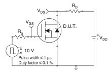
Fig. 10a - Switching Time Test Circuit
