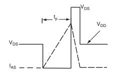
Fig. 12b - Unclamped Inductive Waveforms
