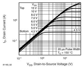
Fig. 2 - Typical Output Characteristics, T<sub>C</sub> = 150 °C
