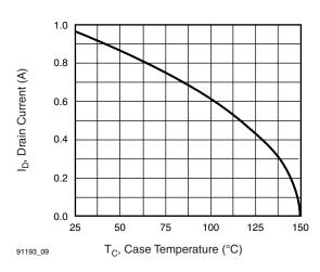
Fig. 9 - Maximum Drain Current vs. Case Temperature
