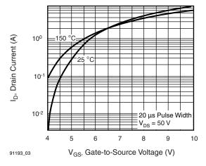
Fig. 3 - Typical Transfer Characteristics
