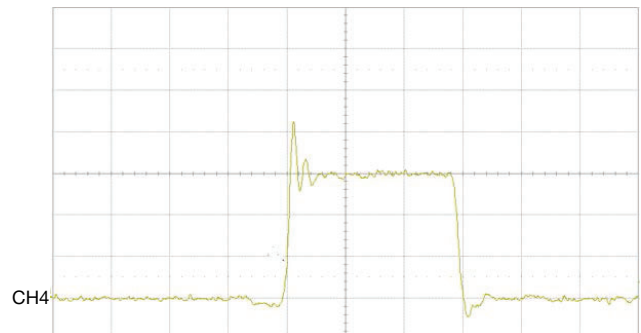
Fig. 20 - Output Switching Waveform CH4 (YLLW) = SW4 (5 V/div.), Time = 10 ns/div.
